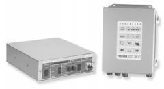
Nexen's web guide controllers & amplifiers provide automatic positioning of the web in response to feedback received from position sensors. They translate information from the sensors into control signals for web position drive motors. The amplifier's motor control output drives an electrical linear actuator to correct the web position by adjusting the roll stand or guide roll mechanism.
